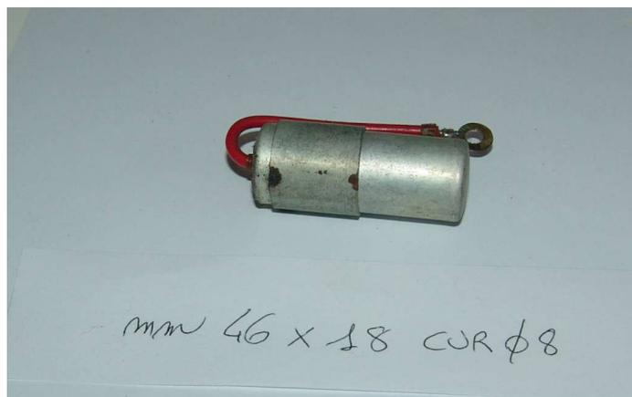
CONDENSATORE CAPACITOR mm 46 x 18 CUR08
