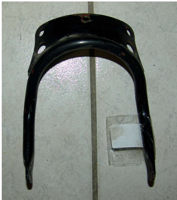
SUPPORTO PARAFANGO POSTERIORE SUPPORT REAR FENDERmorini
