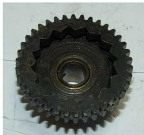
INGRANAGGIO AD INNESTO MESSA IN MOTO MV TR 125 (B356)
