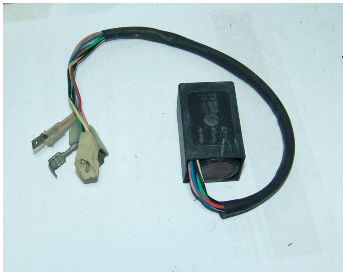
CENTRALINA CONTROL UNIT ??? MORINI 350 CA873
